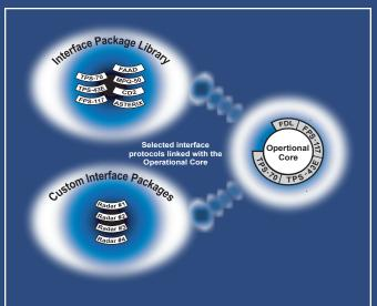
The Interface Package Library (IPL) is a risk reduction technology providing an object-oriented suite of protocol translation packages which can be easily integrated with an Operational Core package to create custom system configurations. IPL packages and the Cores are implemented using the Ada programming language ensuring high reliability and reusability.
