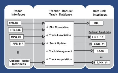
**URIU** normally configured as single workstation supporting multiple data link and radar interfaces. The number of external interfaces supported by a single workstation is virtually unlimited . When more external interfaces are required, the URIU configured can as а distributed network supporting multiple integrated workstations
