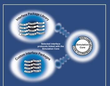
The Interface Package Library (IPL) is a risk reduction technology providing an object-oriented suite of interface protocol packages which can be easily integrated with a Simulation Core package to create custom system configurations. IPL packages and the Cores are implemented using the Ada programming language ensuring high reliability and reusability.
